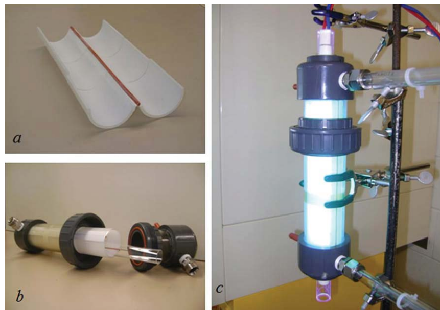
Figure 2. TiO 2 -coated U-shape annular reactor used in the experiments.
